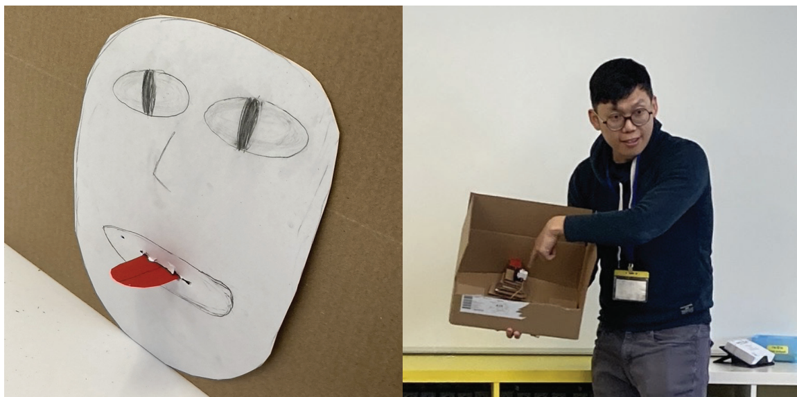
Figure 4.13: During a class discussion, tech teacher Ricardo highlighted the problem solving steps Grade 6 student Ryan followed to make the tongue of his puppet move in and out using the Linear Motor.
